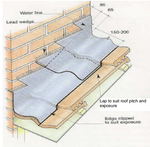
Figure 2 Step flashing to pitched roofs.
